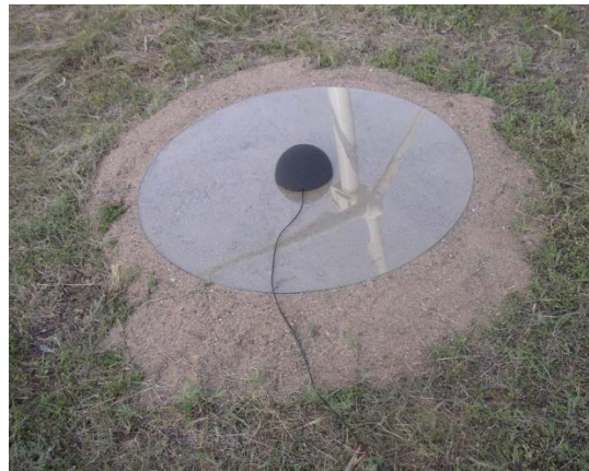
Figure 5: Image of directivity array microphone mounting
